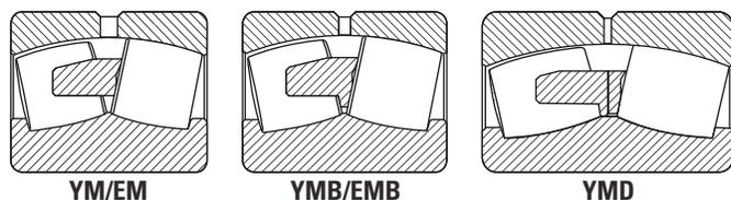
Fig. 6. Machined cages.
