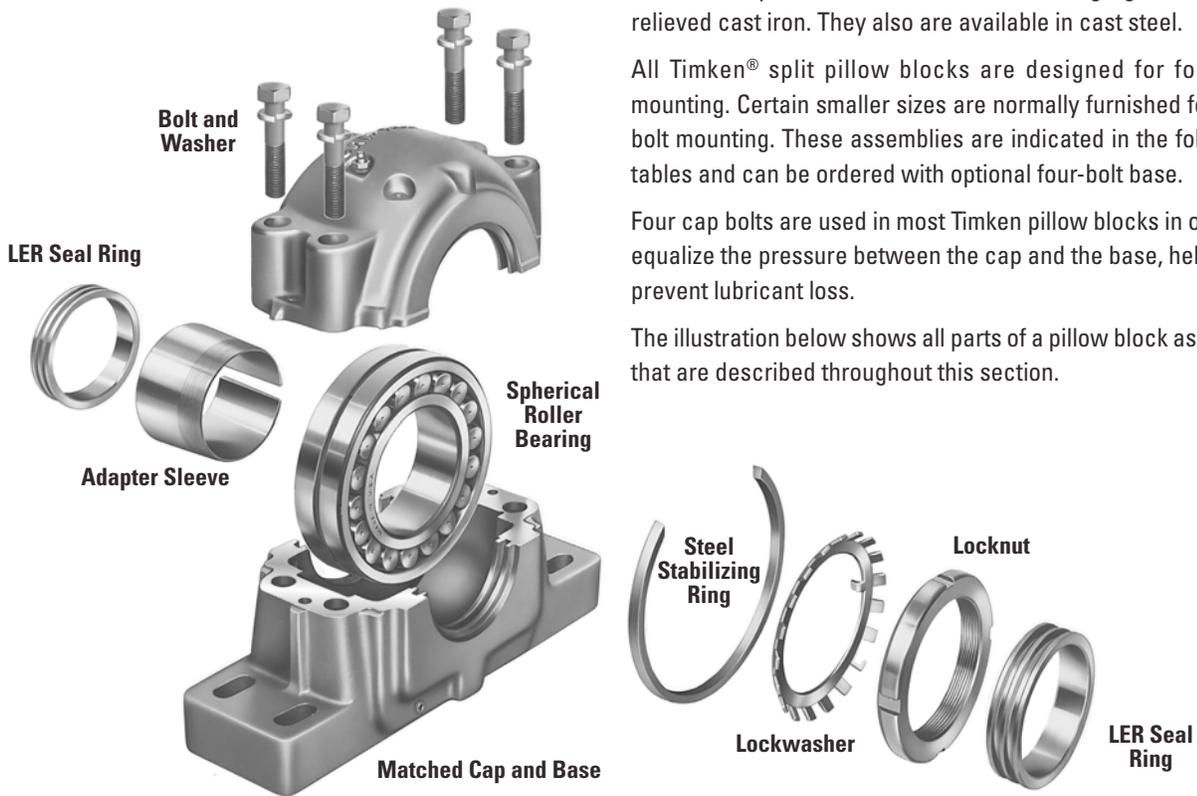
**Fig. 26. Exploded view of a Timken spherical roller bearing pillow block, showing tapered bore spherical roller bearing, adapter sleeve, locknut and lockwasher, stabilizing ring and triple-labyrinth seals. Also shown are recesses in cap and base that form pry-tool slot, and integral fulcrum lugs in base and cap.**
