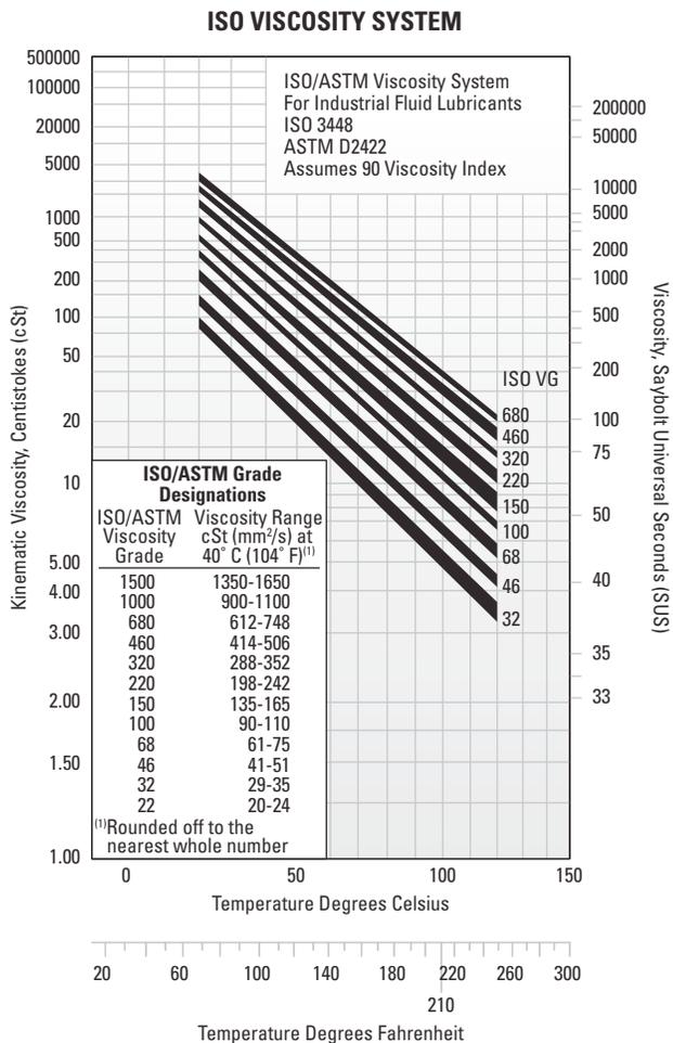
Fig. 20. Viscosity grade system for industrial oils.
