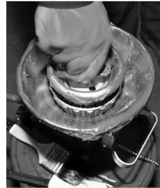
**Fig. 22. Mechanical grease packer.**
