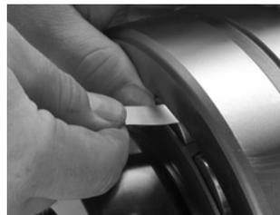
**Fig. 14. Measure RIC before installation.**
