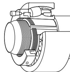
Fig. 32. Hydraulic nut used to withdraw a push-type adapter sleeve.
