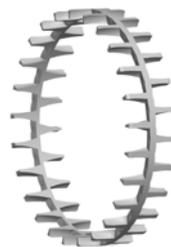
Fig. 7. One-piece, machined-brass, roller-riding, finger-type cage.
