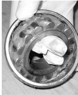
**Fig. 21. Grease can easily be packed by hand.**
