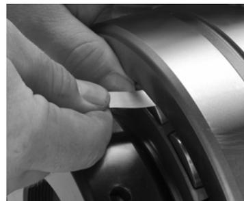
Fig. 18. Measure RIC before installation.
