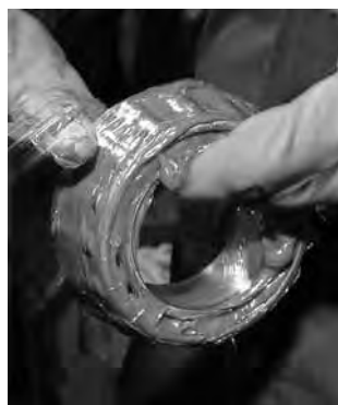
Fig. 14. Grease can easily be packed by hand.
